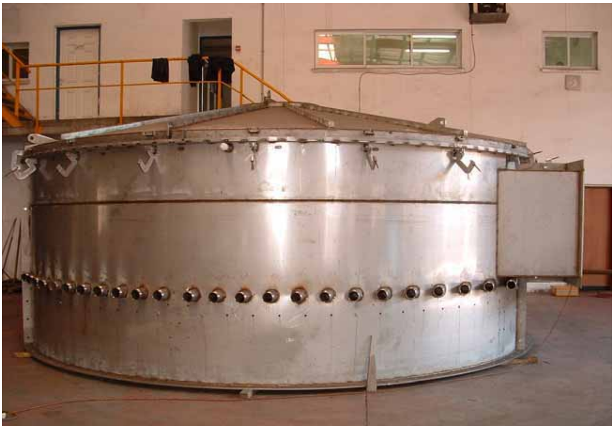
Parts of cyclone filter during manufacturing at our plant application : soy dryer filter. Complete unit is \varnothing 6m 15 m high, 1,920 m 2 filtration area made of stainless steel 304. Unit sent and installed at a soy plant in Ningbo China
